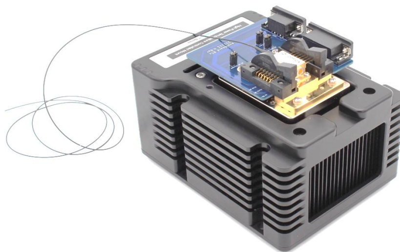
Figure 5 Evaluation Board at Arroyo 264-BB LaserMount
